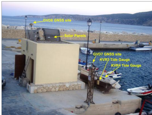
Figure 2 The main facility with its instrumentation setting, called “Theophilos” in Gavdos and the calibration site at the harbor.
