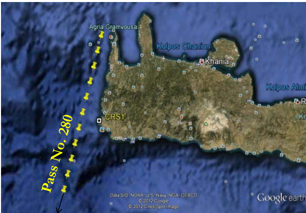
Figure 10. The descending Pass No. 280 of the Chinese altimetric satellite HY-2 in west Crete. The calibration site CRS1 has been prepared for the calibration of this satellite. The IGDR data have already received for Cycles No. 19-22; (19 June-14 Aug, 2012) have been received and preparations are under way for providing the first HY-2 altimeter bias results.
