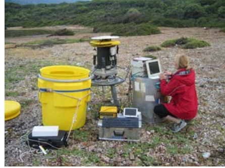
Fig. 4: DIADEM deployment. To determine the geodetic position the GPS antenna was put on the lens. For the astro-observations it was removed.
