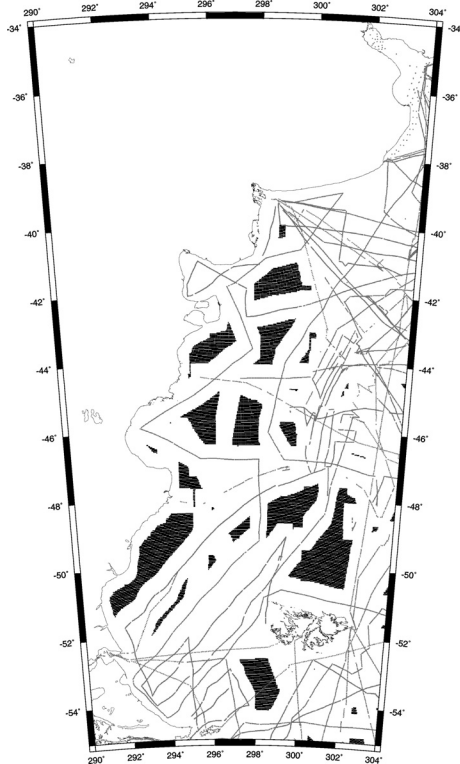
Fig. 1: Distribution of shipborne (gray) and KMS01 (black) data in the area under study.
